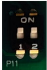
Note: The DIP switch is ON upward and OFF downward
