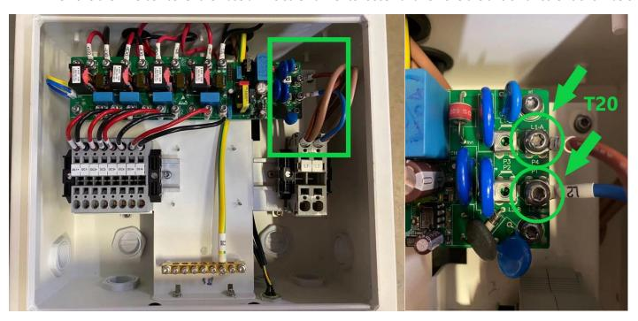
2. Tape off the ends of the blue and brown wires with wire tape so they do not come into contact with anything. Then stuff the wires out of the way, the transmitter is now disabled. The wire box cover can now be reinstalled.
