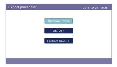
c. Backflow Power is how much power the system is allowed to export to the utility. To set up the system for minimum export, change this value with the Up and Down buttons to read "+00000W" and then press Enter. In order to get maximum export, change this value until it matches the output rating of the inverter. For example, a 7.6K inverter means that Backflow Power should be "+7600W" and a 10K would be "+10000W".
