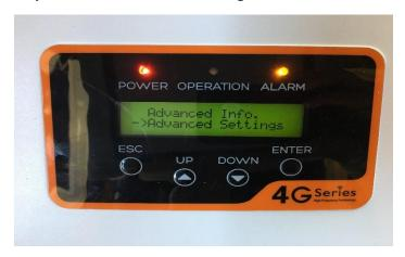
Step 3: Grid On/OFF and set Grid to OFF
